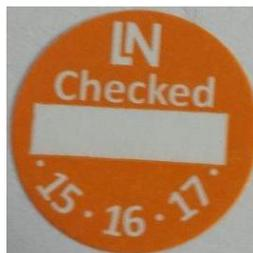
The year of manufacture/shipment and the inspector's initials appears on this test seal.
