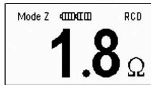
Figure 3.21: Impedance Downstream from an RCCB (brief)
