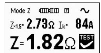
Figure 3.14: Sample Results for Impedance Measurement (detailed representation)
