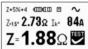
Figure 3.19: Measured Impedance + Measuring Error
