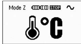
Figure 3.11: Overheating Display After Pressing the Start Key
