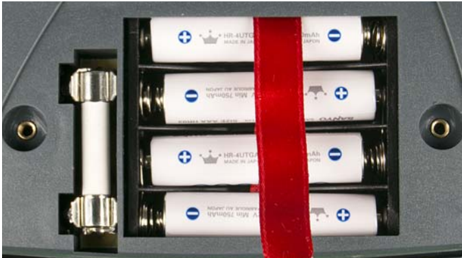
Figure 6.1: Correct Battery Polarity
