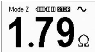
Figure 3.10: Overheating Display – STOP Symbol
