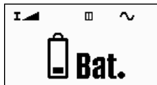
Figure 3.9: Battery Status After Pressing the START Key
