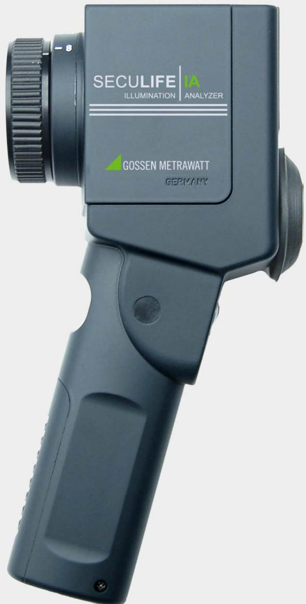
The SECULIFE IA is a high-precision measuring instrument with a measuring angle of 1°. Luminance measurements at distances of 1 meter to infinity can be performed with the instrument. The SECULIFE IA features mirror reflex optics with a 15° field of view, a sharply marked 1° measuring circle at the center and a focusing mechanism.
