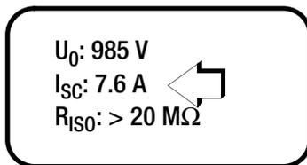
The (+) and (-) terminals at the solar module are short circuited during the measurement, and momentary short-circuit current is measured. Insulation resistance is measured at the same time (see section 9.4).
