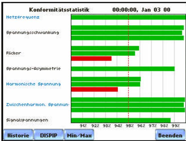
Figure 1: EN50160 Conformity Statistics Provided by MAVOWATT 30/40/70
